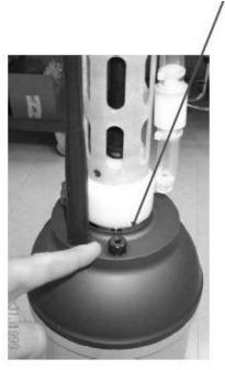
rotate counter -clockwise to unscrew plug.
